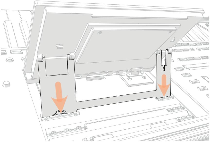
5 Release the **UNLOCK** button to fix the display to the current position.
