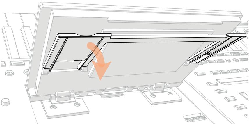
4 While still keeping the **UNLOCK** button pressed, adjust the tilt angle, and fix the bracket to one of the stops in the bottom of the display housing.
